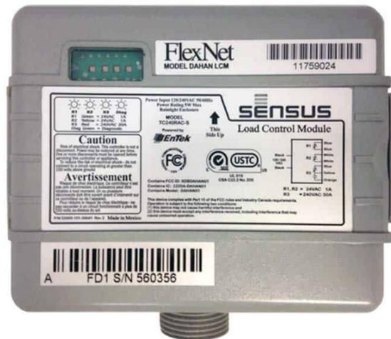
Exhibit 5 (Flexnet Load Control Module (LCM) Data Sheet).
